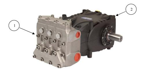
Left to right shaft conversion is an easy operation that takes minutes to be accomplished. Turning the manifold and the back cover up-side down are the two operations required to change crankshaft side.
