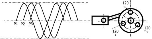
To be noted that the reciprocating motion of the plungers, consistent with the crank mechanism design, produces three pulsating waves P1 P2 P3 that translates into a flow rate of pulsating nature.
